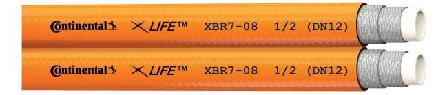
XBR7 is a **medium-pressure, twin-line thermoplastic hydraulic hose**. Known for its flexibility and high abrasion resistance, this hose is compatible with petroleum, water and synthetic-based fluids. Applications include mobile equipment, lube lines, blowout preventers, hydraulic lifts and construction machinery.
